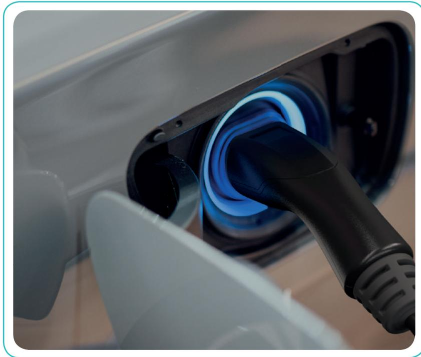
Cable equipped with Type2 - EU connector
